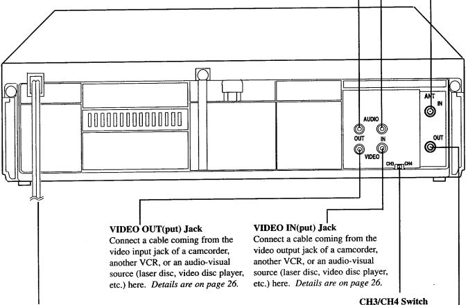
**AC Power Cord** Connect to a standard AC outlet to supply power to the VCR.
